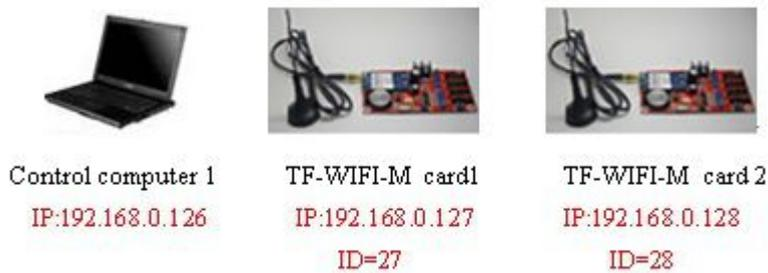
1、 Check the name and password of the router using a single network cable connected to a wireless router, enter the router to see (on the back of the router has IP, username, password), connect the TF-WF-M card 1, installed antenna, power, turn on the computer Wi-Fi, and find the control card WIFI name, click on the link, as shown below
