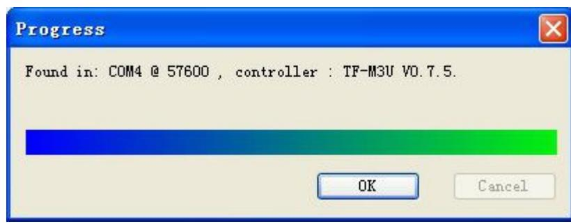
It shows that the communication between control card and computer is o
