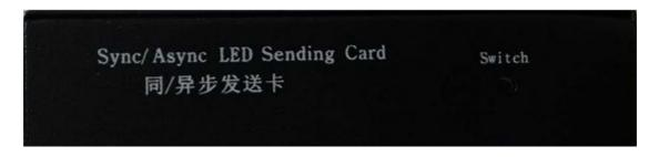
Switch: Switch Sync and Async, press this button 2 seconds then release.
