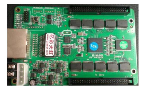
YC\_LC105 card contains 2 Ethernet ports. Either one can work with
