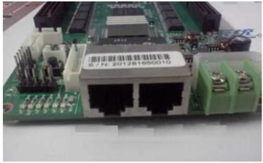
One end of the Ethernet cable connects to YC\_LC105 card. The other end insert
