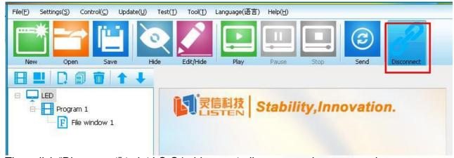
Then click "Disconnect" to let LS-Q1 video controller as asynchronous mode;
